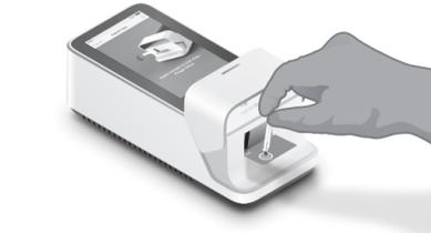
Sample application using a transfer tube
