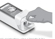
Sample application using a transfer tube
